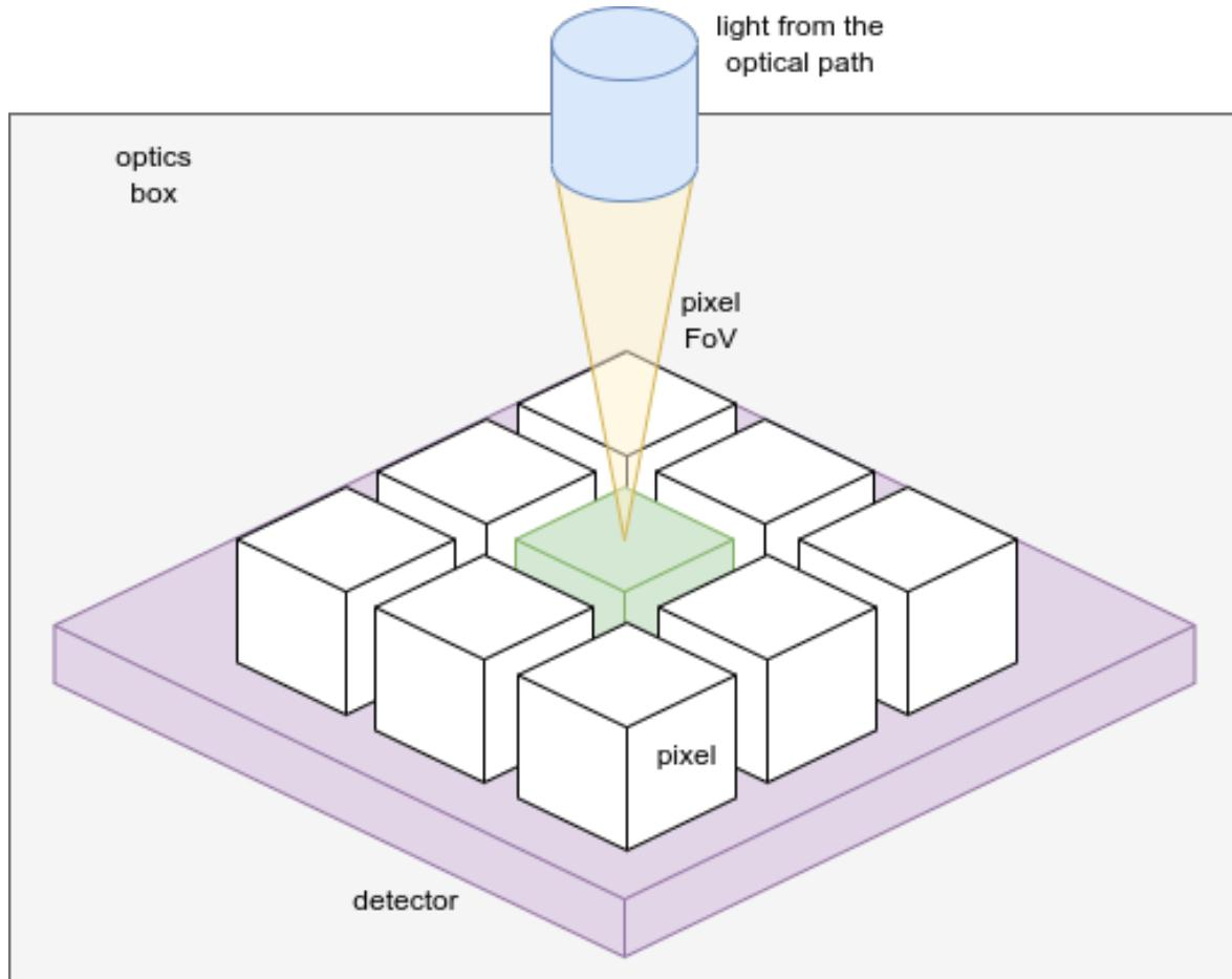
The image summarize the problem. The green detector is illuminated by the yellow cone from the optical path. The optics box, represented in gray, irradiates it from the top, except from the yellow cone, and hence  $\pi - \Omega_{pix}$ . The detector box, in purple, irradiates the pixel from the back:  $\pi$ .
