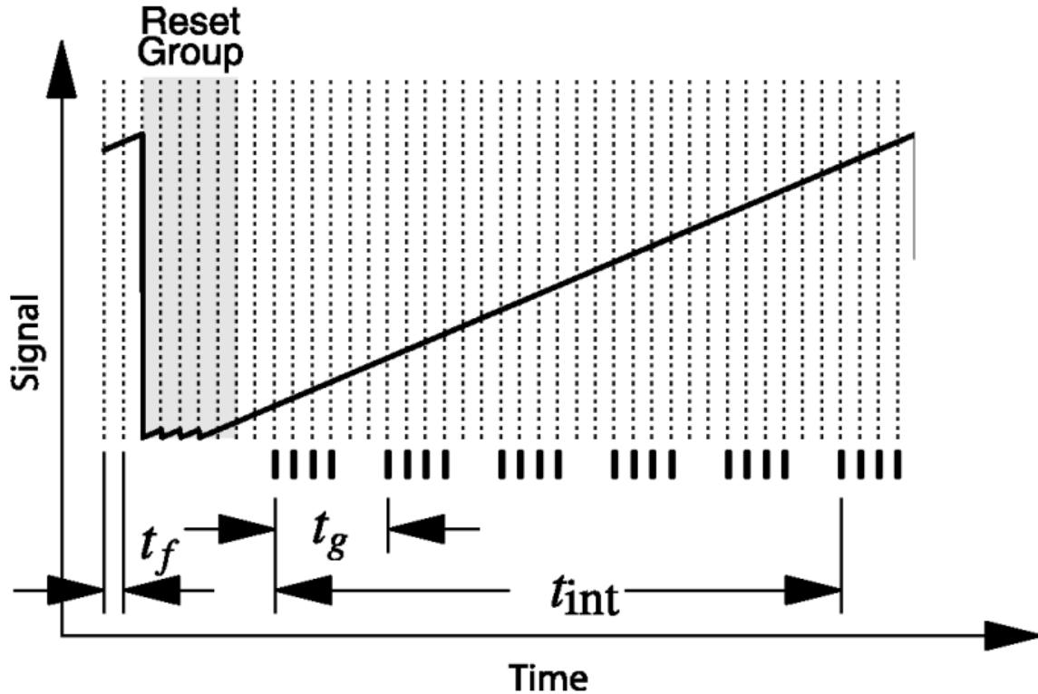
The picture from Rauscher and Fox et al. 2007 (<http://iopscience.iop.org/article/10.1086/520887/pdf>) shows the detector readout scheme using MULTIACCUM sampling. The detector is read out at a constant cadence of  $t_f$  but not all the read frames are saved. Saved frames are averaged, resulting in one averaged group of data every  $t_g$  seconds.
